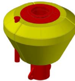
Buoyant particular showing moon pool for multiparameter probe to collect bio-chemical data, ADCP and further sensors.
