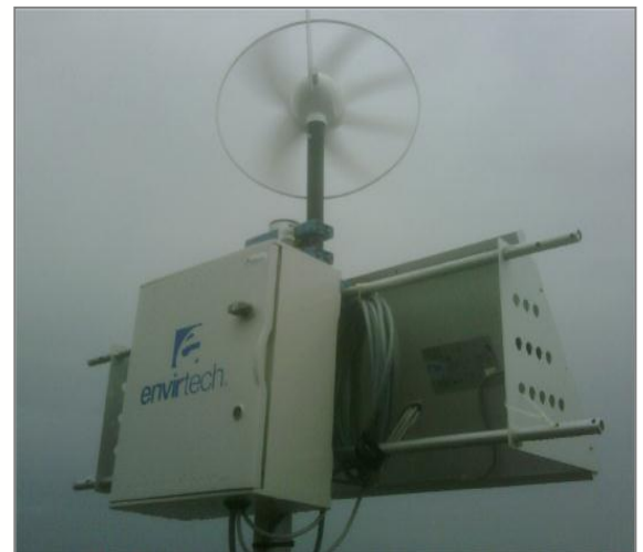
The eTide-I/T in Venice Laguna, Malamocco South Gate (Italy), powered by solar panel and eolic generator.
